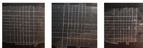
Fig. 5: Cross-Cut Test of Dual-Cure PUA systems
